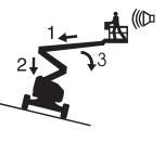
Do not operate the machine in strong or gusty winds. Do not increase the surface area of the platform or the load. Increasing the area exposed to the wind will decrease machine stability.
