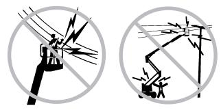
Maintain required clearances from electrical power lines and apparatus in accordance with applicable governmental regulations and the following chart.
