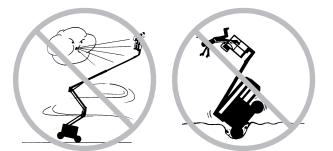
Use extreme care and slow speeds while driving the machine in the stowed position across uneven terrain, debris, unstable or slippery surfaces and near holes and drop-offs.
